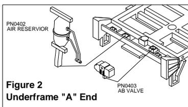
**Step (2).** Place Accumate coupler (PN0120) into the coupler box (PN0019). Install the coupler lid (PN0020), and attach the assembly to the underframe (PN0369) using the short screw (PN0100).
